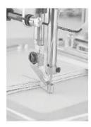
Foot leverage amount and pressure could be modified using the touch screen panel, no particular tools required.
